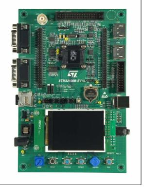
With a complete range of hardware evaluation features, the STM32100B-EVAL board is designed to help developers evaluate all device peripherals (such as HDMI CEC, motor control, LCD, microSD Card™, serial Flash, speaker, IrDA and USART) and develop their own applications.
