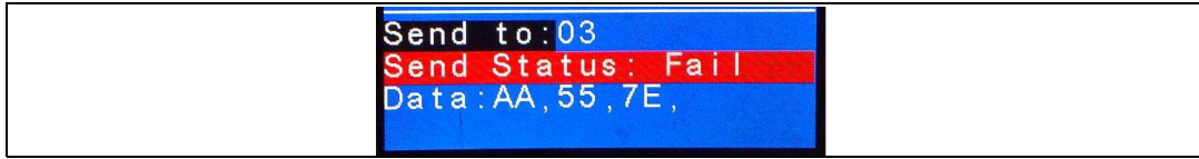
Figure 8. LCD screen shot of a failed send transaction
