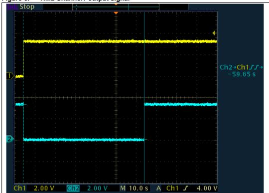
Figure 6. TIM2 Channel1 output signal
