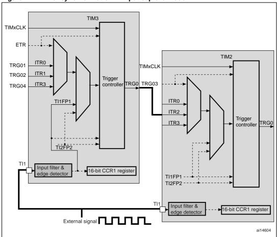
Figure 2. Timer synchronization in input capture mode
