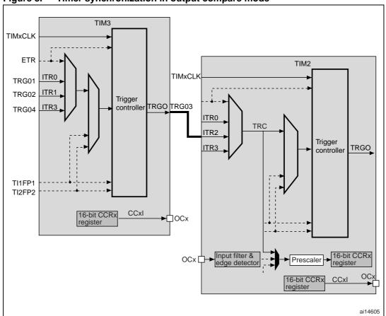
Figure 3. Timer synchronization in output compare mode
