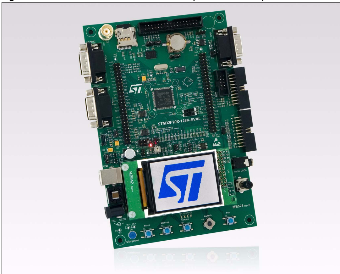
Figure 1. STM32F10X 128 K evaluation board (STM3210B-EVAL)
